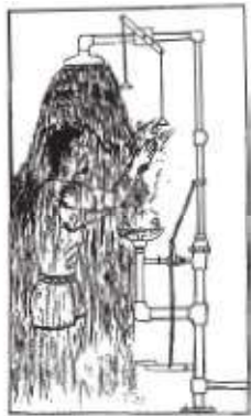
FIG 6.18: EMERGENCY SHOWER AND EYE WASH FOUNTAIN
